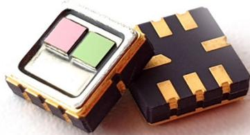
We are proud to present our new **SMD type** dual channel thermopile sensor preferably intended for NDIR gas analysis. Heimann Sensor is the market leader in thermopile arrays and sensors. With our patented thermopile technology, we are able to produce very fast thermopiles and fully monolithic thermopile arrays with high signal and high specific detectivity.
